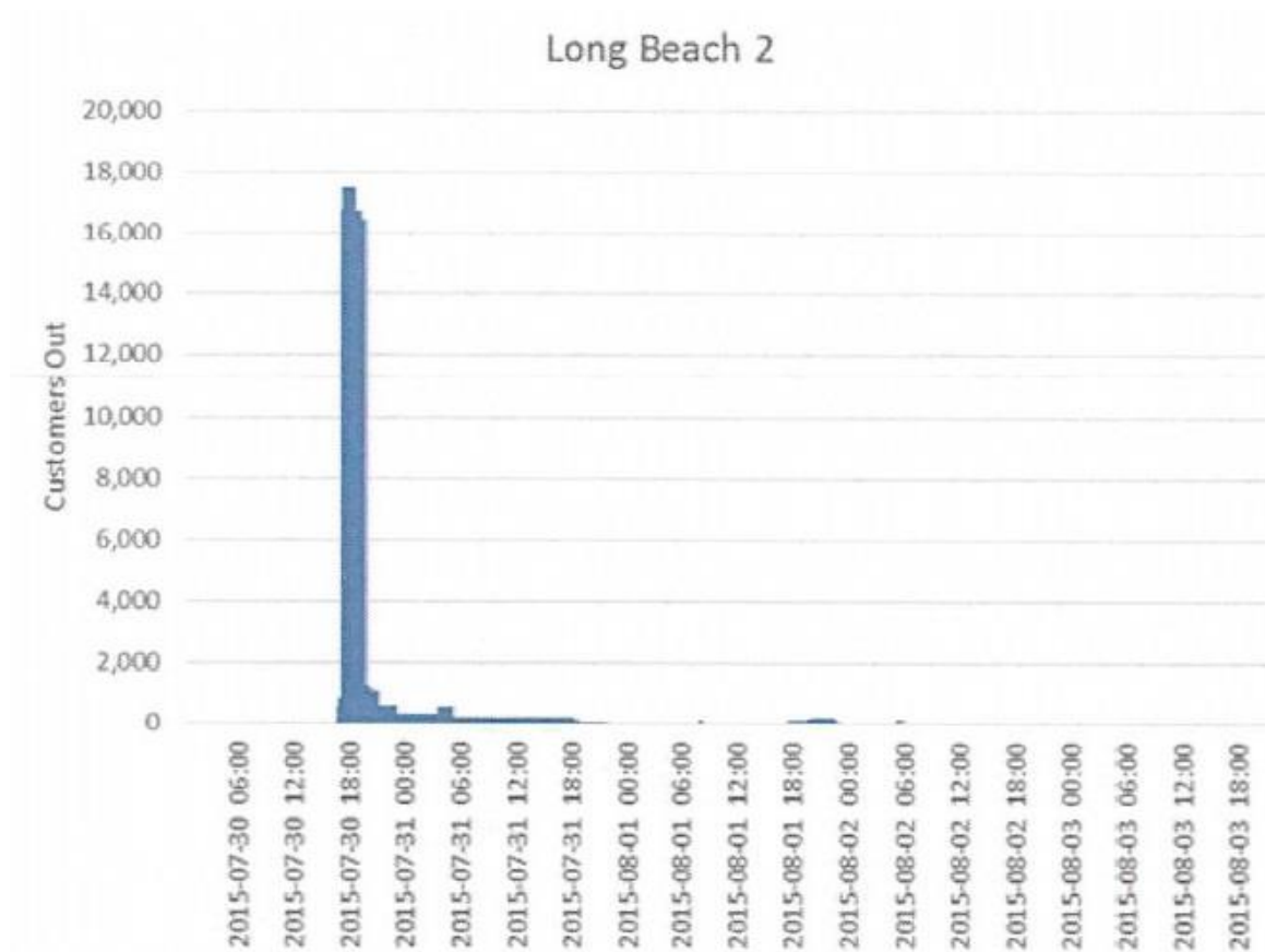
Figure 8: Number of customers out by date and time for July 30-August 3, 2015 outages. The small customer outages after 00:00 hours on August 1, 2015, represent repairs and restoration activities for the final few customers. Source: Davies Consulting.
