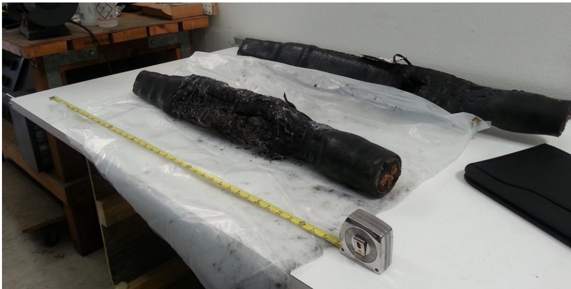
Figure 6: Float 12kV (front) and Steam 12kV (rear) PILC splices. Source: CPUC
