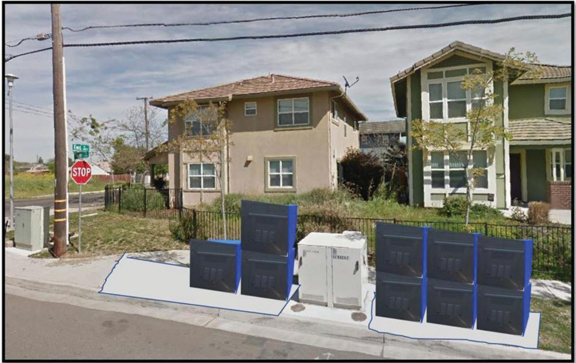
A permanent generator would require a 100-gallon propane tank on a 300 square foot footprint.<sup>83</sup> This option is also infeasible given the constraints of the average ROW.
