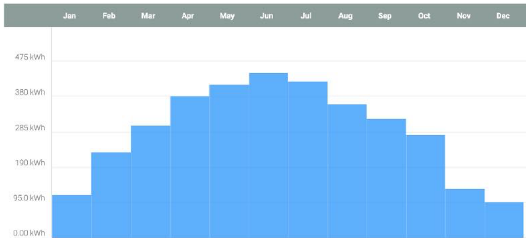
Figure 24. System Monitoring Report from a Typical Residential Solar System 221
