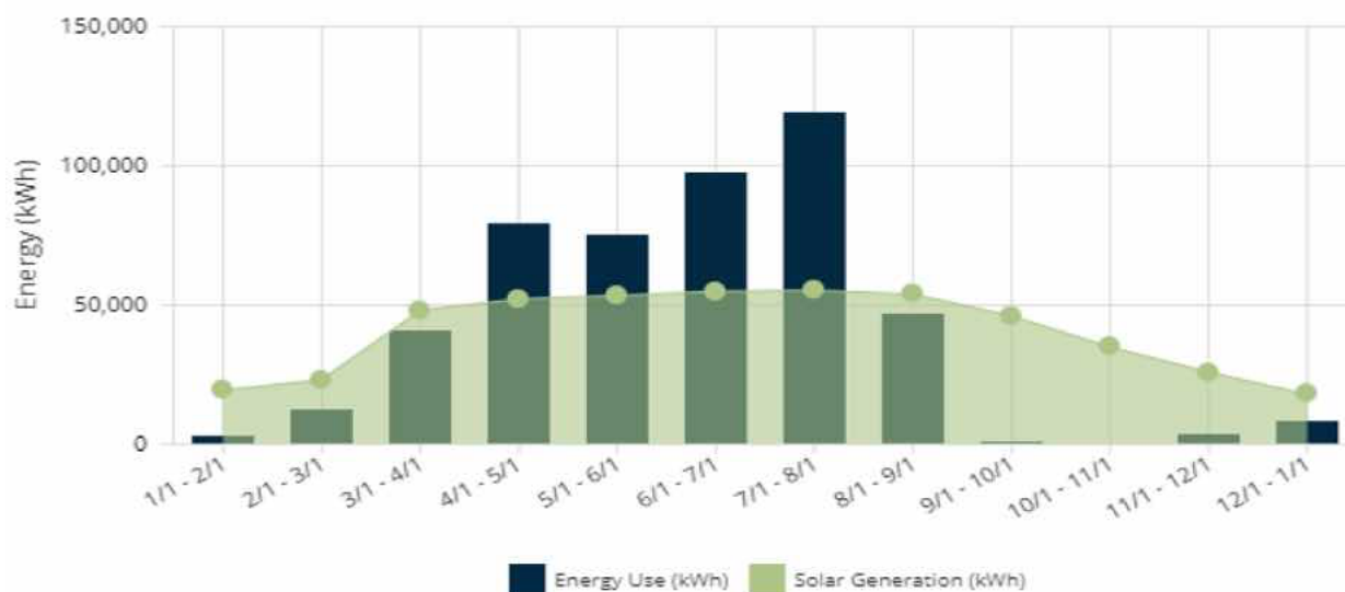
Figure 12. Energy Use and Solar Production for a Deep Irrigation Well
