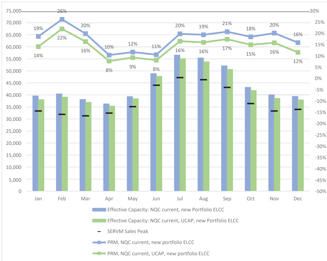
Figure 7: Comparison of monthly PRM under current NQC counting, with the new solar, wind, storage, and hybrid portfolio ELCC, and with UCAP for CCs and CTs
