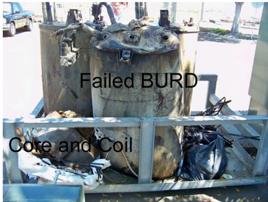
Figure II-6 D2 (BURD Transformer): Catastrophic Failure
