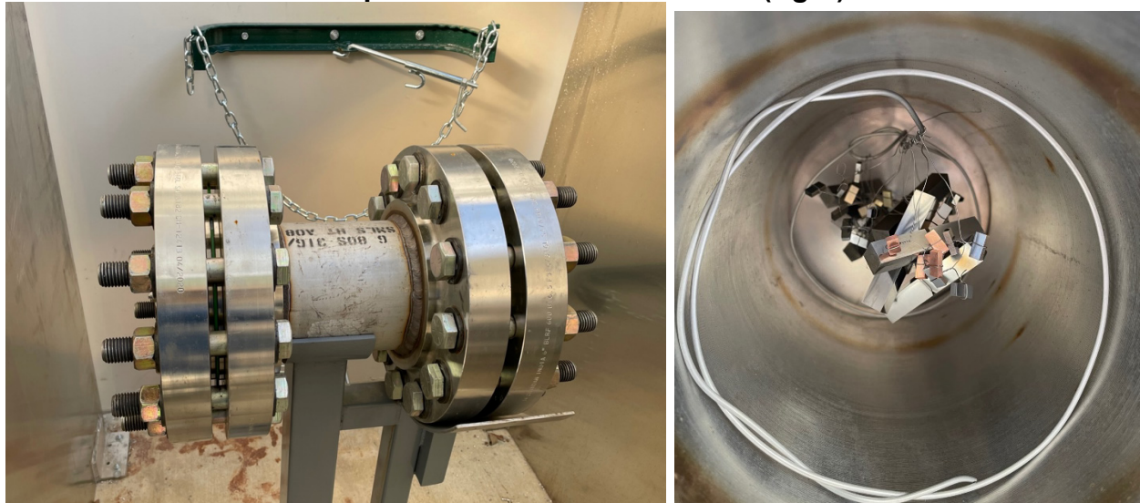
Figure 83: View of Test Chamber with Heating Element and Thermal Insulation
