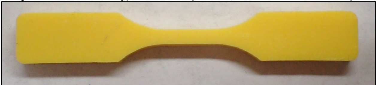
Figure 40: ASTM D638 Type-V Tensile Specimen, Die Cut from Molded Plaque
