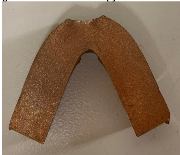
Figure 109: Photo of Charpy Tested Cu Alloy
