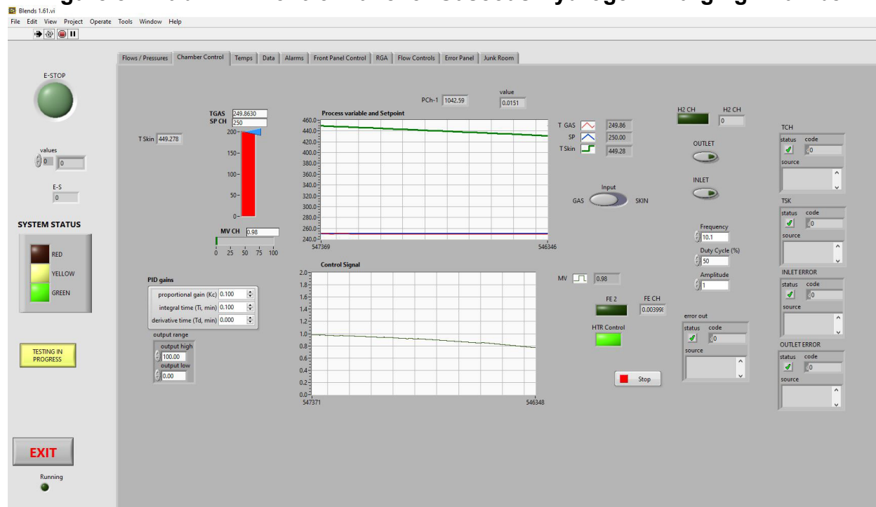
Figure 84: LabVIEW Control Panel of Gaseous Hydrogen Charging Chamber
