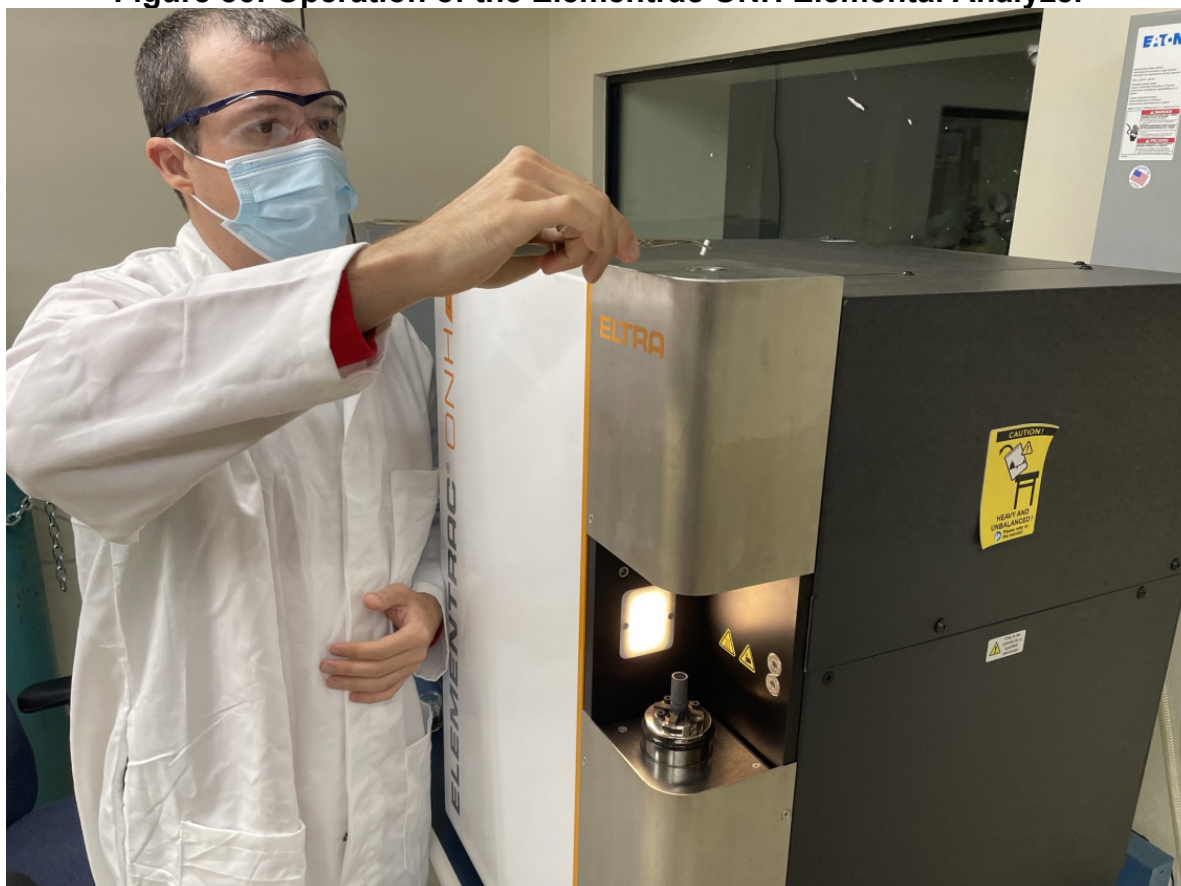
Figure 85: Operation of the Elementrac ONH Elemental Analyzer
