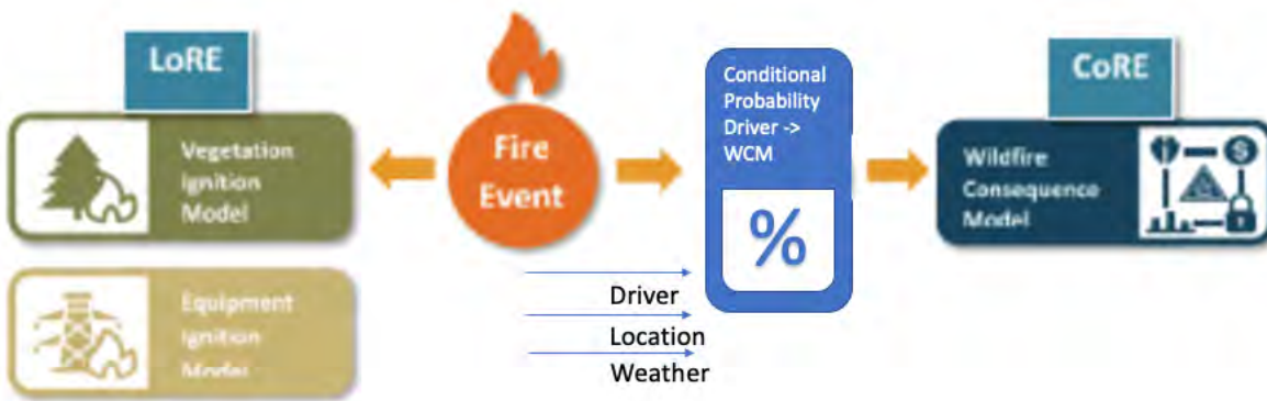
Figure 6 - The risk model can be corrected by applying a conditional probability that corrects for the fact that not all fire drivers are as likely to create an ignition on the worst fire weather days. Sophistication of the approach can be enhanced by additionally adding location and weather data.
