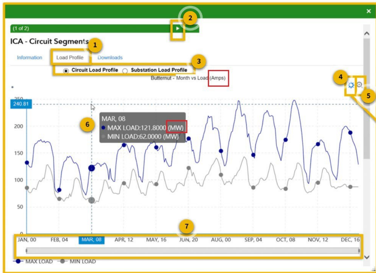
Figure 6-8: Screen capture of SCE's user guide (Oct. 9, 2023) with a title suggesting that results are presented in Amps but data labels showing MW.
