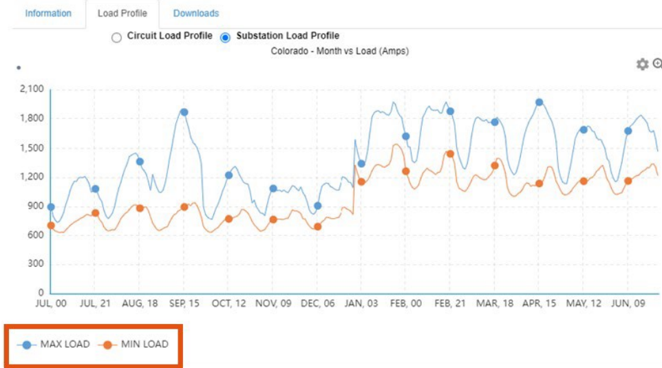
Figure 6-13: Screen capture of load profile for the Colorado Substation for SCE (Oct. 14, 2023). Orange box indicates where language is not aligned with recommendation.
