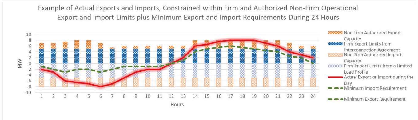
Figure 9: Example of Actual Exports and Imports Constrained between Authorized Operational Limits and Minimum Export and Import Requirements
