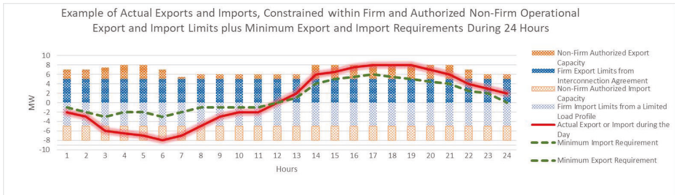
Figure 16: Example of Actual Exports and Imports Constrained between Authorized Operational Limits and Minimum Export and Import Requirements
