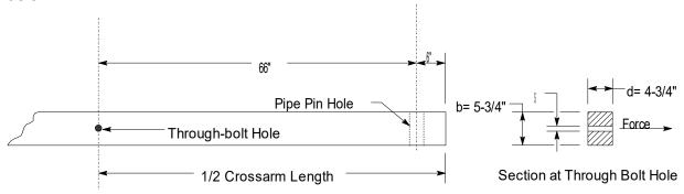
The section through the arm and the method of computing the fiber stress is shown below. Note: for simplicity this example only assesses weak axis bending stress on the crossarm, there may be other load effects that should be assessed.
