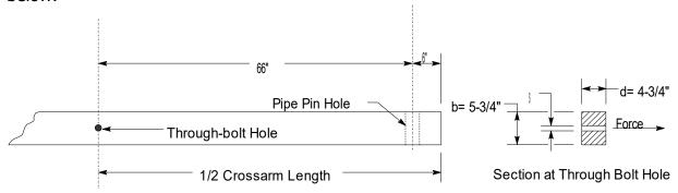
The section through the arm and the method of computing the fiber stress is shown below.
