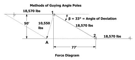
Assuming the pole height and framing as shown in Part 2, the top circumference of pole to be 25", the ground circumference to be 50" and the center of load to be 37.4 feet above ground line (as determined in Part 2), the fiber stress on the pole at the ground line is as follows:
