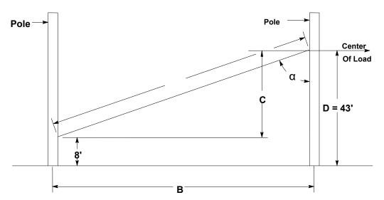
The head guy should be attached approximately at the normal center of load, therefore:
