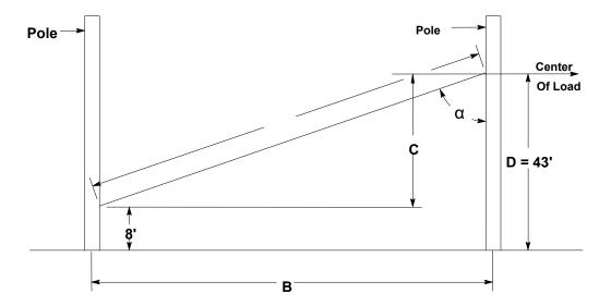
The head guy should be attached approximately at the normal center of load, therefore:
