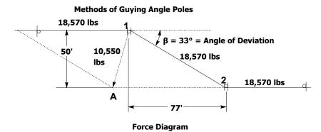
Assuming the pole height and framing as shown in Part 2, the top circumference of pole to be 25", the ground circumference to be 50" and the center of load to be 37.4 feet above ground line (as determined in Part 2), the fiber stress on the pole at the ground line is as follows:
