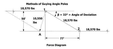
Assuming the pole height and framing as shown in Part 2, the top circumference of pole to be 25", the ground circumference to be 50" and the center of load to be 37.4 feet above ground line (as determined in Part 2), the fiber stress on the pole at the ground line is as follows:
