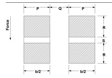
The method of calculating the unit fiber stress of the double crossarms acting as a simple beam is as follows:
