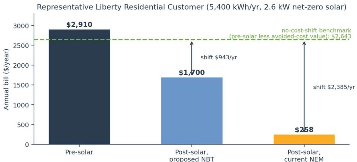
Figure B-1. Annual bills for the representative Liberty residential customer. The dashed benchmark is the pre-solar bill less the avoided-cost value of the system's output; the distance below it is the cost shift to non-participants.
