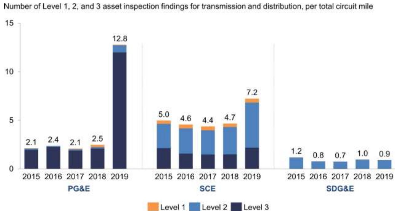
Figure 2.1a: Asset inspection findings normalized by total circuit mileage (Large utilities)
