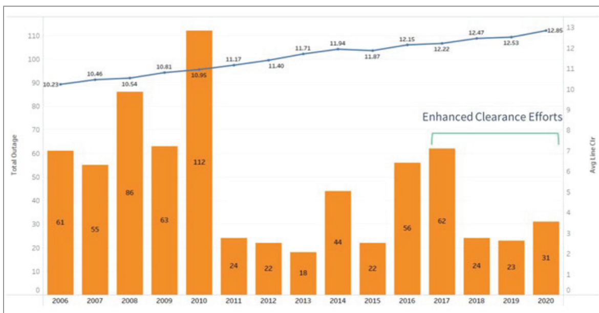
Figure 4.6.5-3: SDG&E Vegetation-Related Outages versus Average Line Clearance 111
