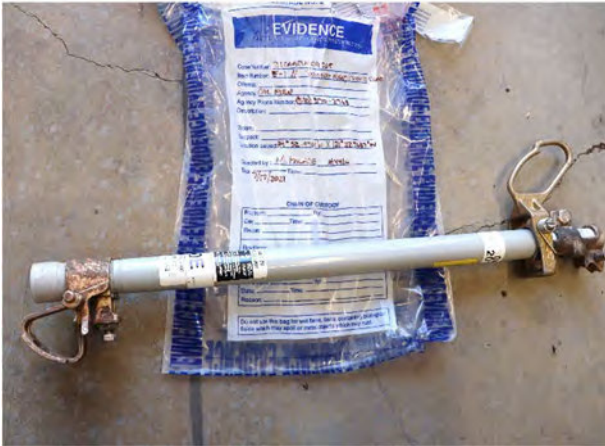
Figure 17: One of two fuses that operated
