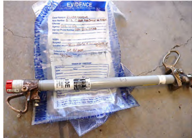
Figure 18: Fuse that did not operate
