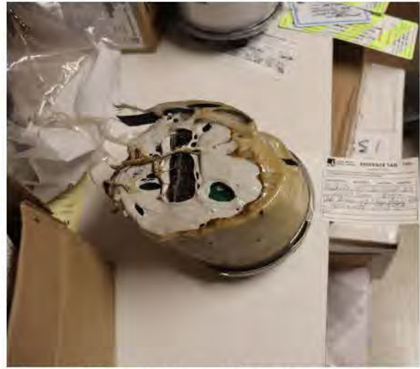
Figure 24: Melted SmartMeter from the Dixie Fire
