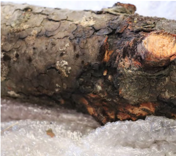
Figure 19: Subject Tree trunk where energized conductor contacted tree.
