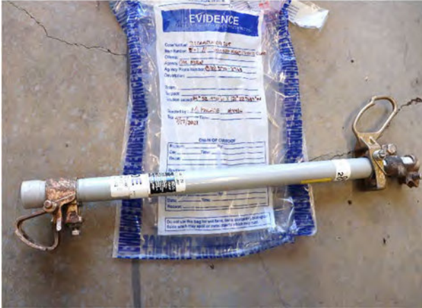
Figure 17: One of two fuses that operated
