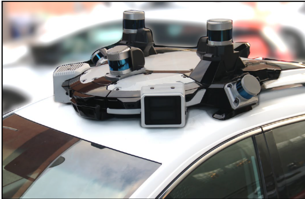
Figure 7. Roof mounted sensor array which includes lidars, cameras, and radars. [REDACTED] [REDACTED] [REDACTED] [REDACTED]
