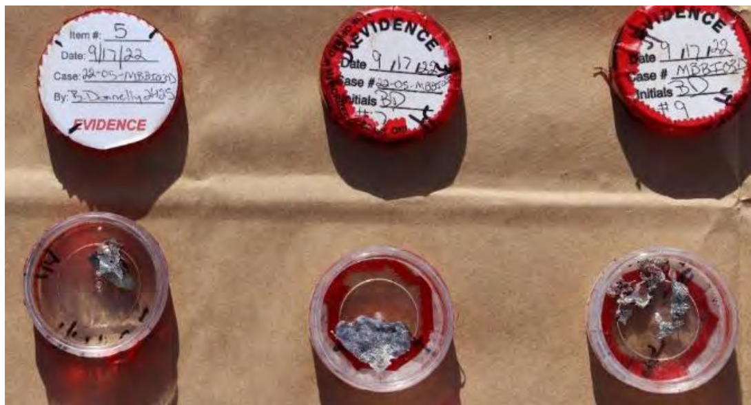
Figure 25: Examples of metallic flakes collected by USFS. 69
