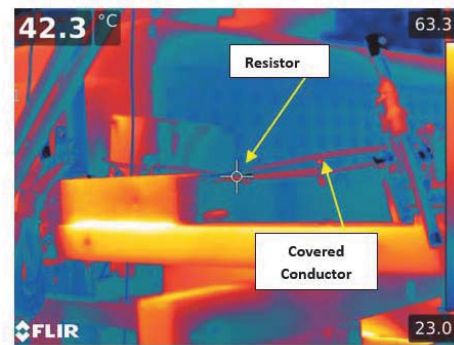
11:13 AM De-Energized –Conductor Temp.: 42.6°C 11:14 AM Energized –Test Subject Temp.: 42.3°C
