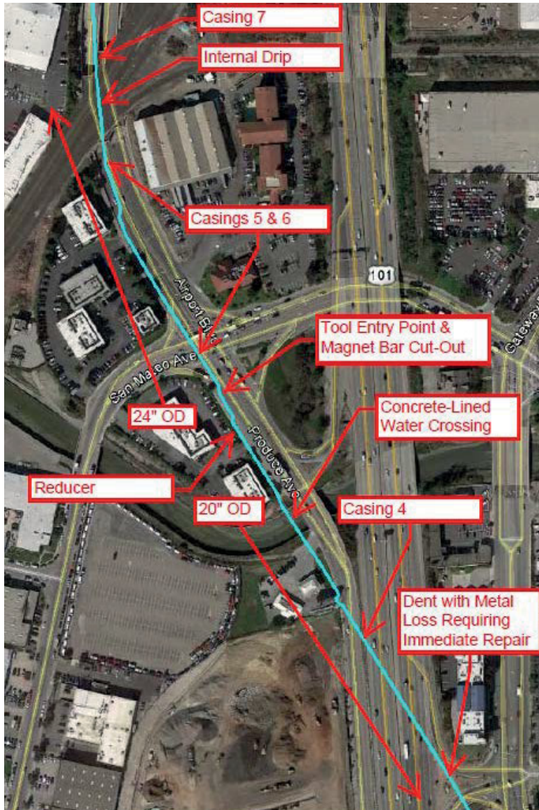
Example of inspection in SF Bay Area [IPC2016-64586]
