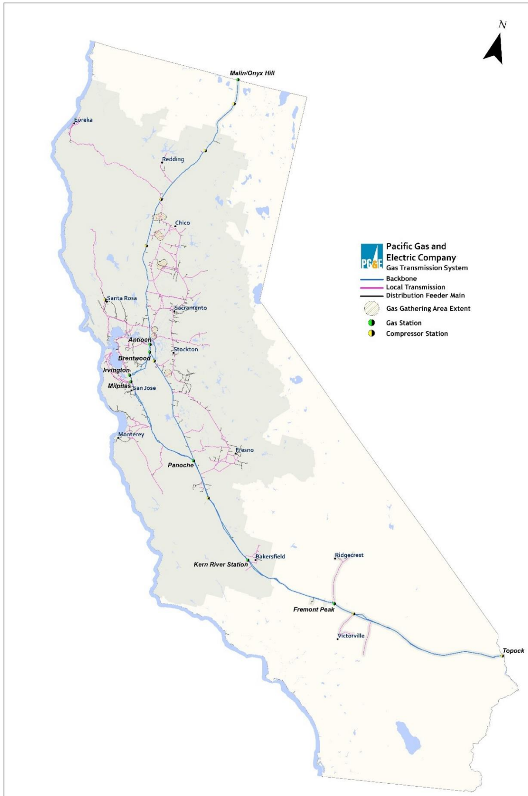
FIGURE 3-2 PG&E CITYGATE: INTERCONNECTIONS BETWEEN PG&E BACKBONE SYSTEM AND LOCAL TRANSMISSION AND DISTRIBUTION SYSTEM
