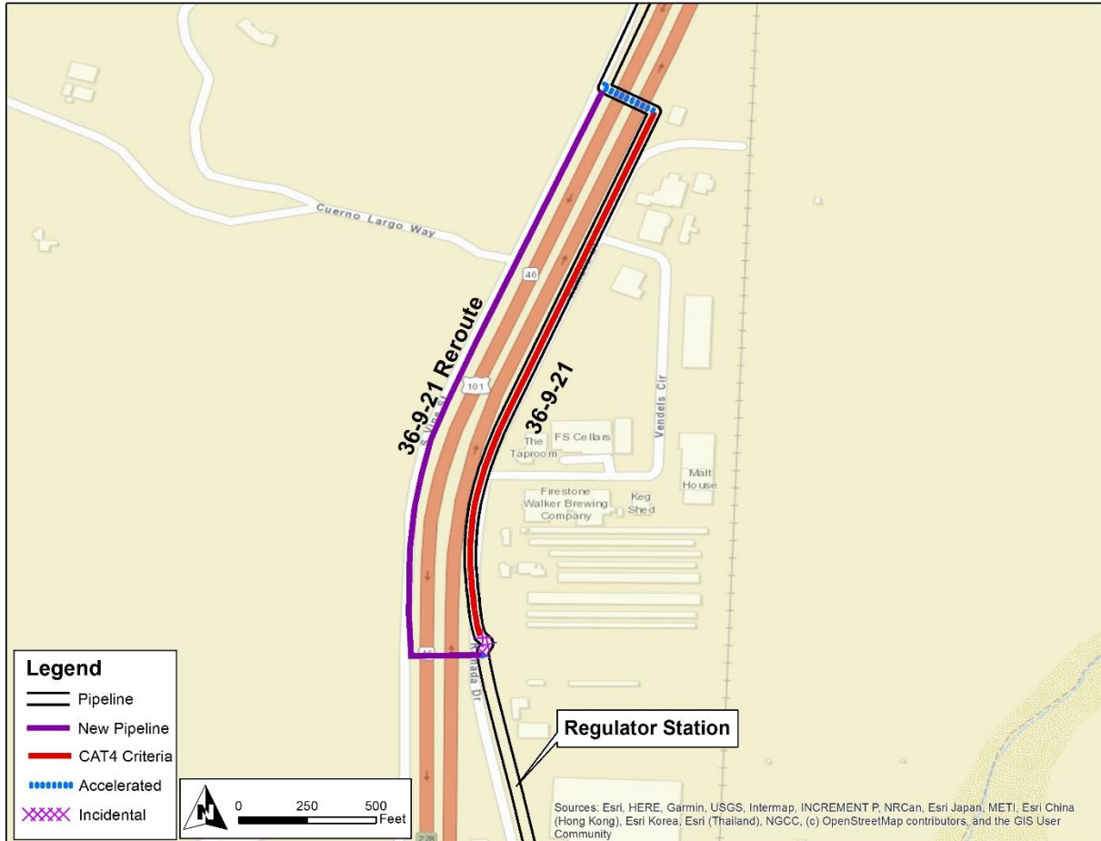
Figure 2: Overview Map of Supply Line 36-9-21 Replacement Project
