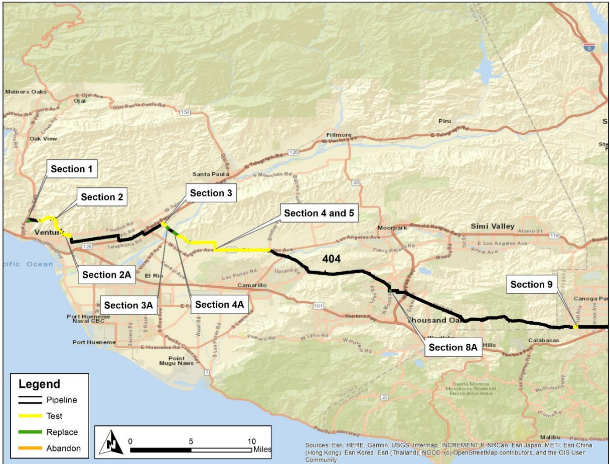
Figure 1: Overview Image of Line 404 Hydrotest and Replacement Projects
