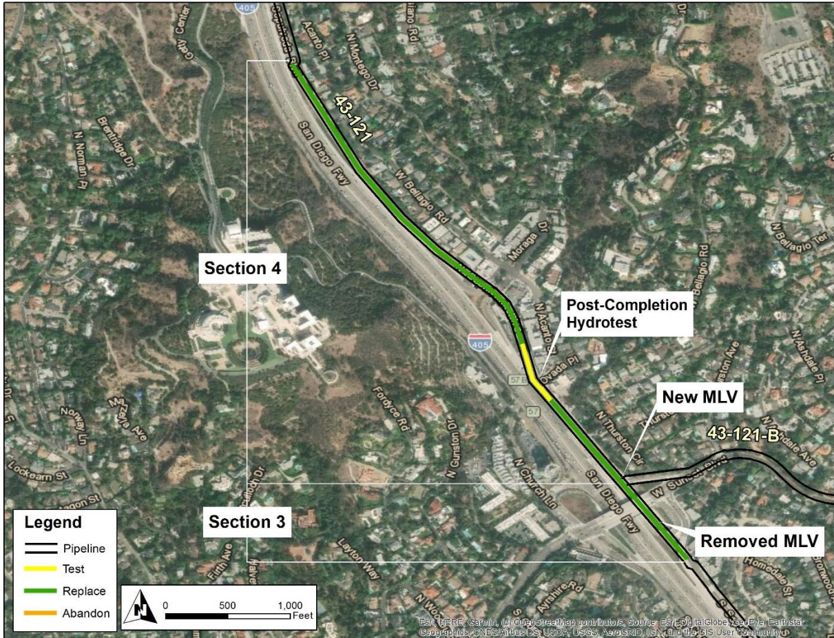
Figure 6: Satellite Image of Supply Line 43-121 North Section 3 and Section 4 Replacement Project
