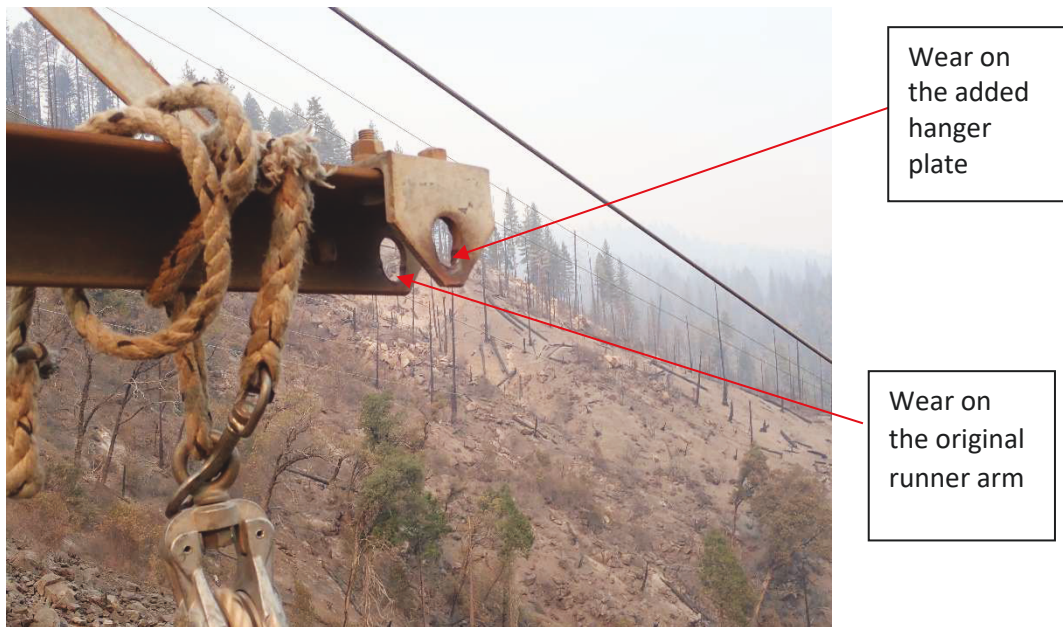
Figure 7. The right runner arm and the added hanger plate from the Incident Tower prior to removal from the tower for evidence. Photo provided by PG&E. 83
