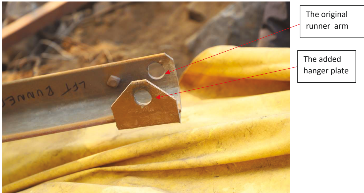
Figure 6. The left runner arm and the added hanger plate from the Incident Tower. 82
