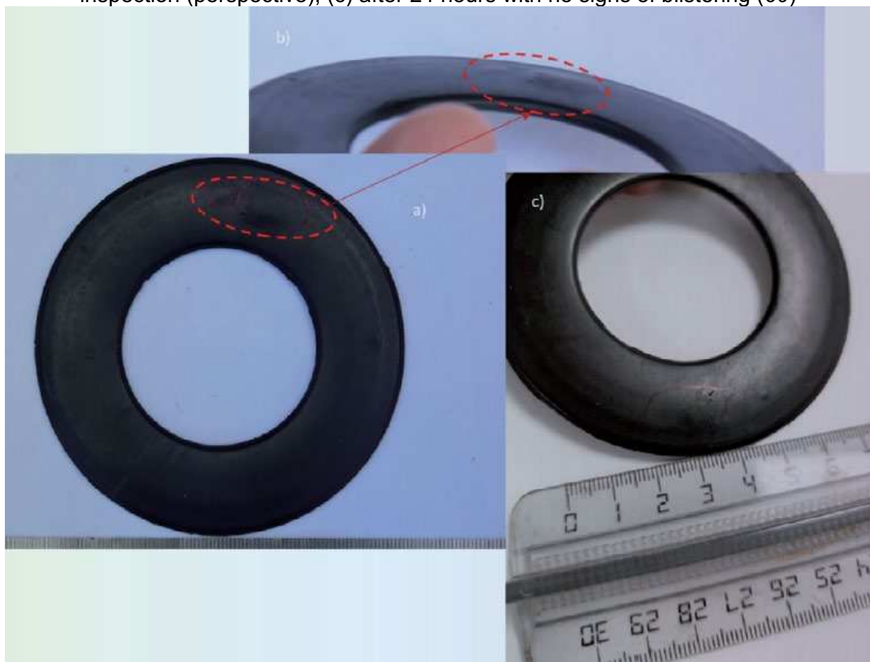
Figure 12: Blistering on seal, observed in (a) immediate inspection, (b) immediate inspection (perspective), (c) after 24 hours with no signs of blistering (60)
