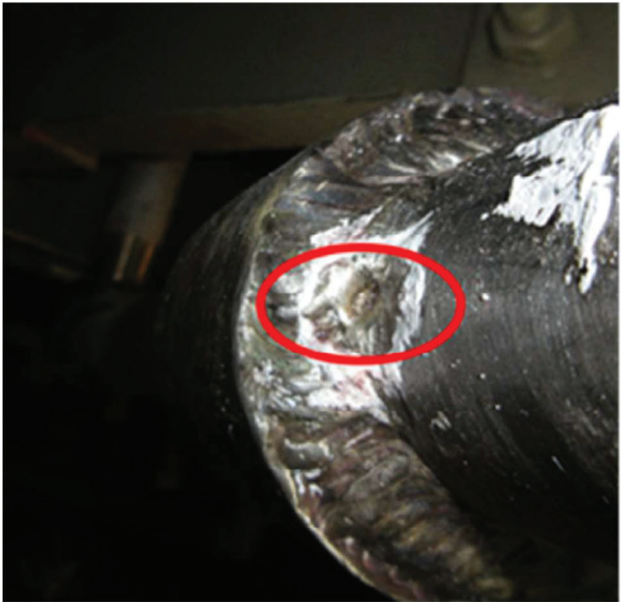
1 Figure 3-11 Weld Defect – Close-up View of Leak Location and Pin-Hole 2 Weld Defect at Coupling Socket Weld 316
