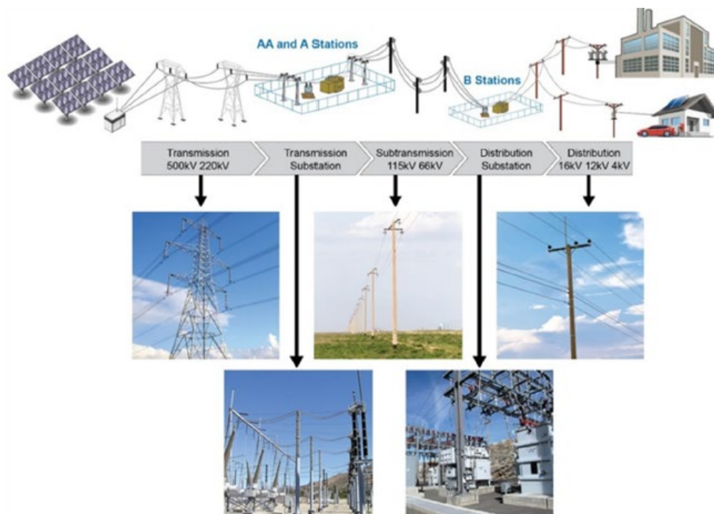
Figure II-3 Electric Grid – Power System Overview
