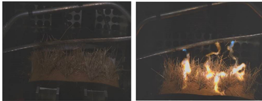
Figure I-27 Arcing from a Downed Power Line Test With (left) and Without REFCL (right)
