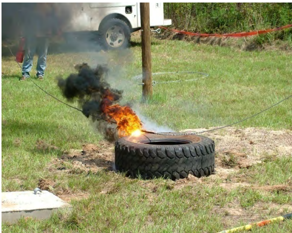
Fig. 7. Dry tire test –generates 15 A fault current immediately
