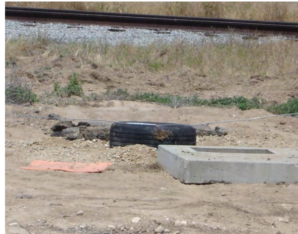
Fig. 6. Wet tire test – no fault current during a 2-minute downed conductor
