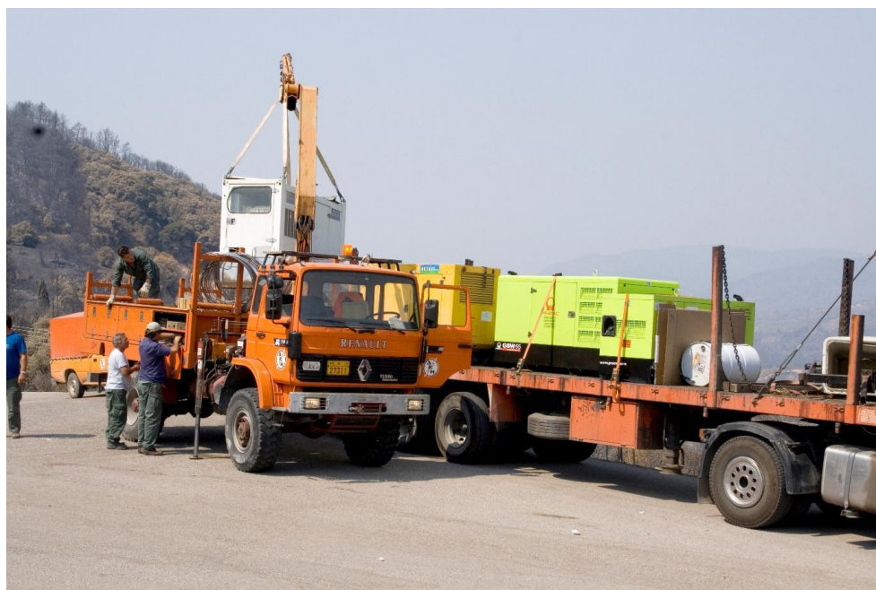
Figure 4: Use of mobile generators for restoration (Courtesy: Public Power Corporation, Greece).
