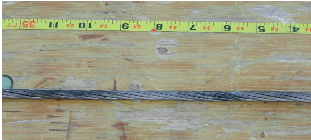
Figure II-2 #4 ACSR Conductor from Koenigstein with Soot Deposits
