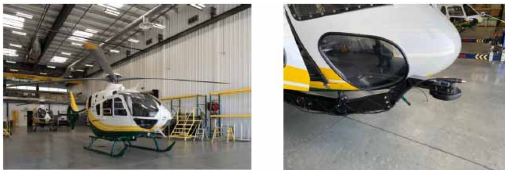
Figure II-18 SCE Helicopters (left) and Mounted with Infrared and Corona Camera (right)
