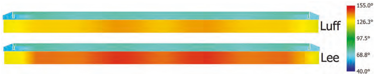
Fig. 1 Temperature distribution on the Luff and Lee side 516 MVA, 0.90 PF with 40 C cold air
