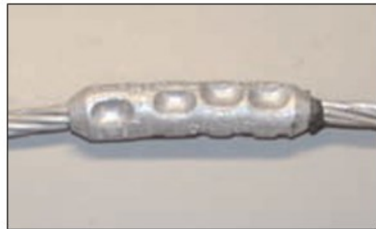
Figure B-81: Compressed Line Splice
