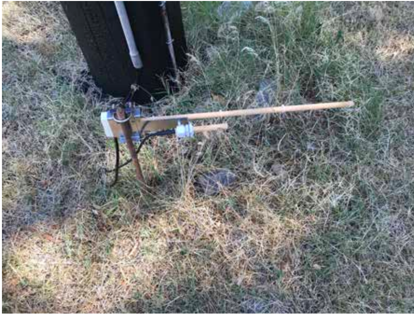
Figure 2—Typical Fuel Monitoring Device
