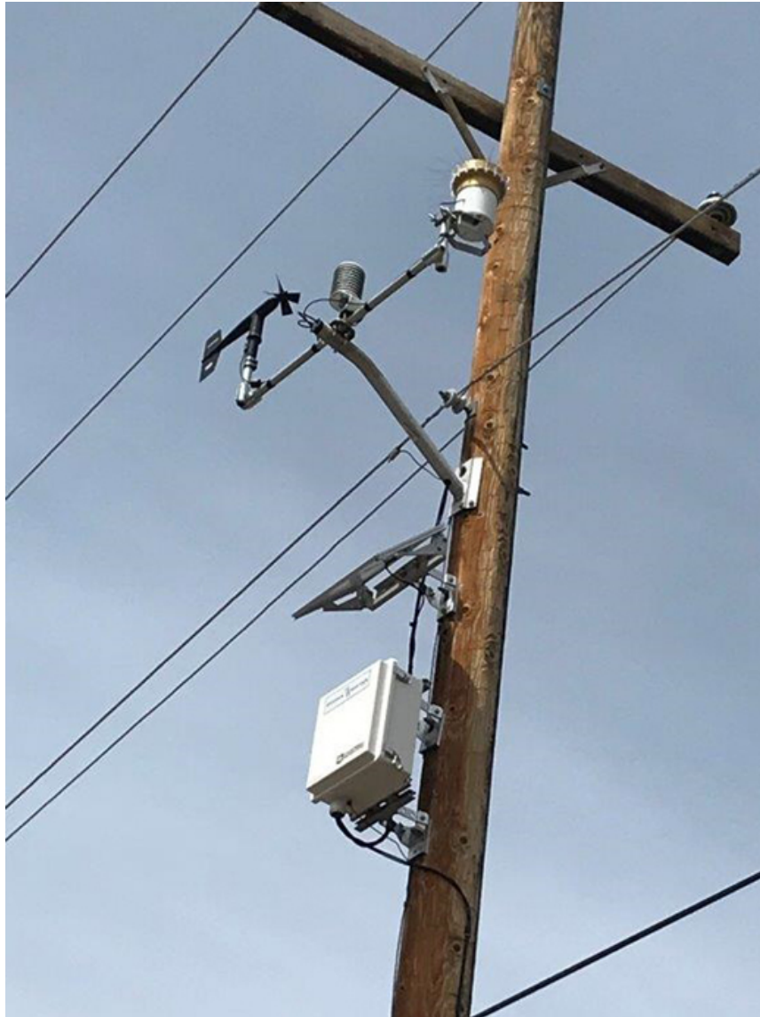
Figure 1—Typical Weather Station Installation
