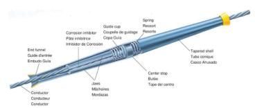
cutaway view. It uses internal compression springs and tension jaws that grip the conductor. There have been a number of overhead splice failures on the PG&E system. A notable example was the splice failure at Candlestick Park
