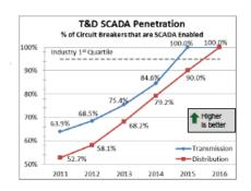
PG&E's saturation is at 58 percent, compared with an overall industry position of over 95 percent. This initiative will continue the SCADA additions underway and bring PG&E to 100 percent by 2016 (except for 4 kV substations).
