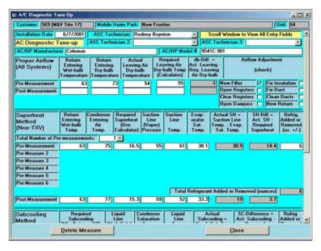
Figure 2. AC Diagnostic Tune-up Data Collection Screen (Superheat and subcooling values and refrigerant properties are checked when data is entered to ensure quality control).
