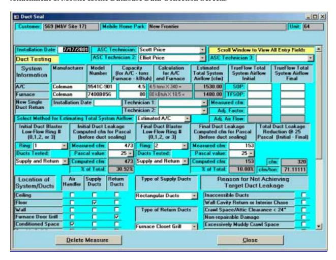
Figure 1. Duct Testing and Sealing Data Collection Screen (Computed cfm and cfm/ton leakage reduction are computed and checked to ensure quality control).
