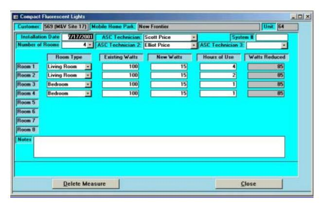
Figure 3. CFL Data Collection Screen (Watts reduced are calculated in database to ensure quality control).
